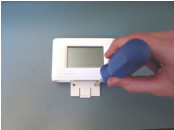
Illustration: Mounting the HUMLOG 10
