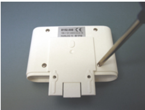
Illustration: Opening the HUMLOG 10 to change the battery
