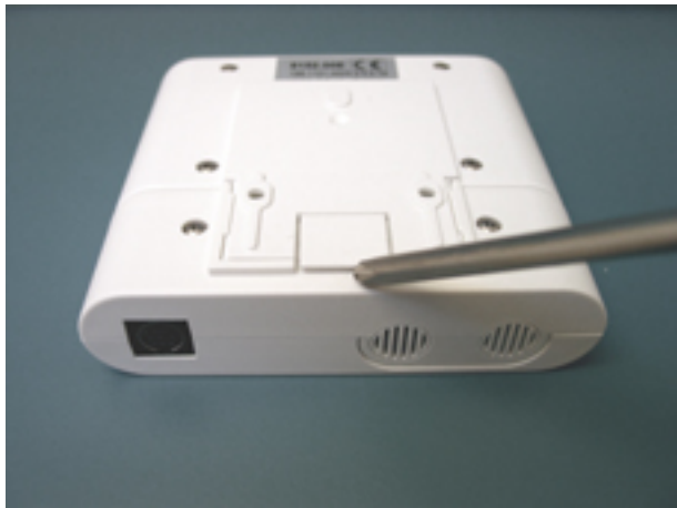
Illustration: Removing the Back-Plate
